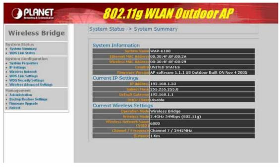
Wireless Bridge mode help to make the two or more Ethernet networks connected without any wire. With multiple WAP-6100s in this mode, several LANs in distance can communicate to each other. This could be deployed if the networks are hard to make the wire in between.
